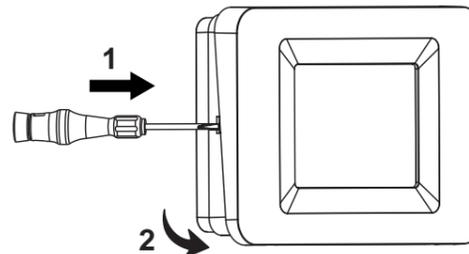
Remove the inner cover over the clamps by unscrewing the retaining screw and turning the cover to the left. Fix the base to the wall, using horizontal (A-B, A-D, A-A) or vertical (C-C) spacing.
