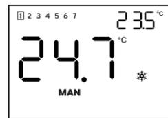
The thermostat regulates the room temperature exclusively according to the manual temperature setting.
