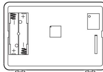
TO CLOSE THE DEVICE, COUPLE THE TWO PARTS AND PRESS THE FRAME OF THE FRONT PART UNTIL THE TWO SIDE HOOKS CLICK.
