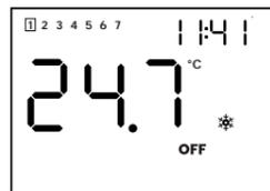
The display shows OFF, the clock and the room temperature. The antifreeze function is active. In this mode the thermostat preserves the system by activating the boiler only when the room temperature drops below a minimum value (factory set at +6°C).
