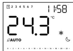
The comfort set temperature (hereinafter: TC) or reduced set temperature (hereinafter: TR) changes automatically depending on the time program stored.
